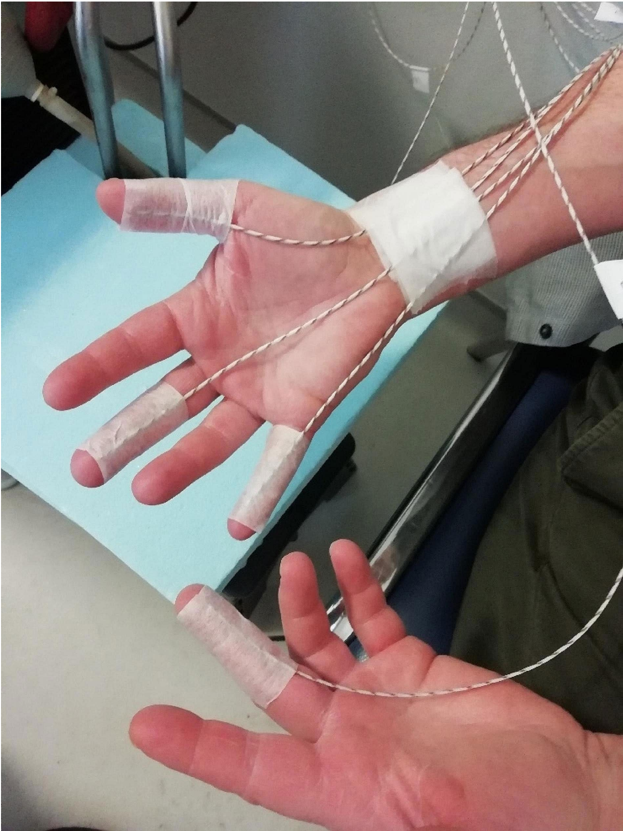
Fig. 2 Installation of the thermocouples
